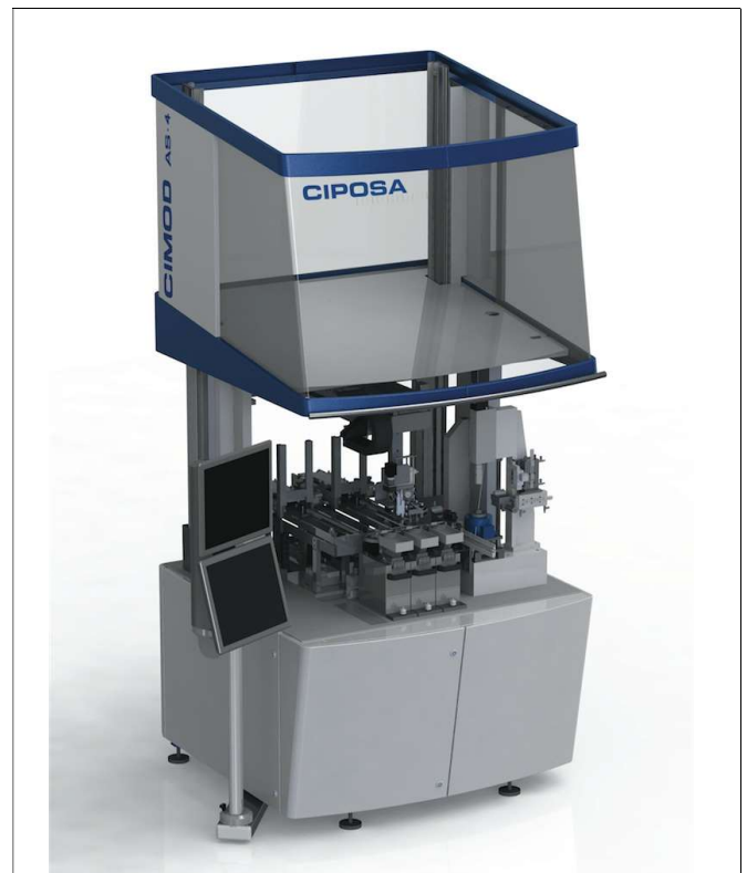
La machine CIMOD AS 4 comportant trois stations.
